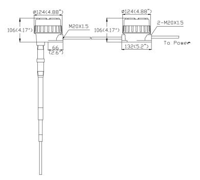
Figure 4.2 AVI-PDU remote system mounting
