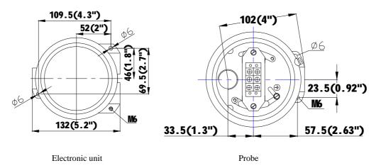
Figure 4.3 XP housing installation
