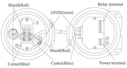
Figure 4.6 Remote System wiring
