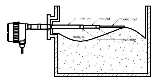
Figure 1.2 Sensing element construction
