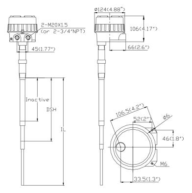
Figure 4.1 AVI-PDU integral system mounting
