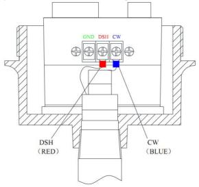
Figure 4.5 Integral System wiring
