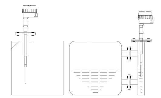
Bracket mounting in open vessel
