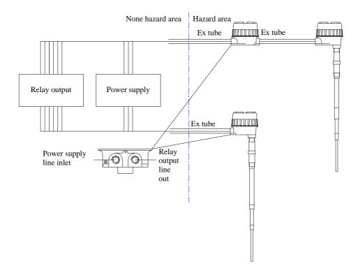
Figure 4.4 System wiring
