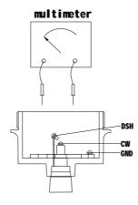
7.2 Testing sensing element
