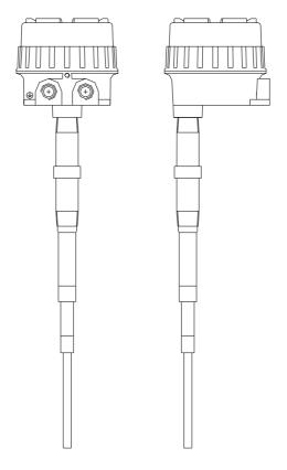
Figure 1.1 AVI-PDU series RF level switch
